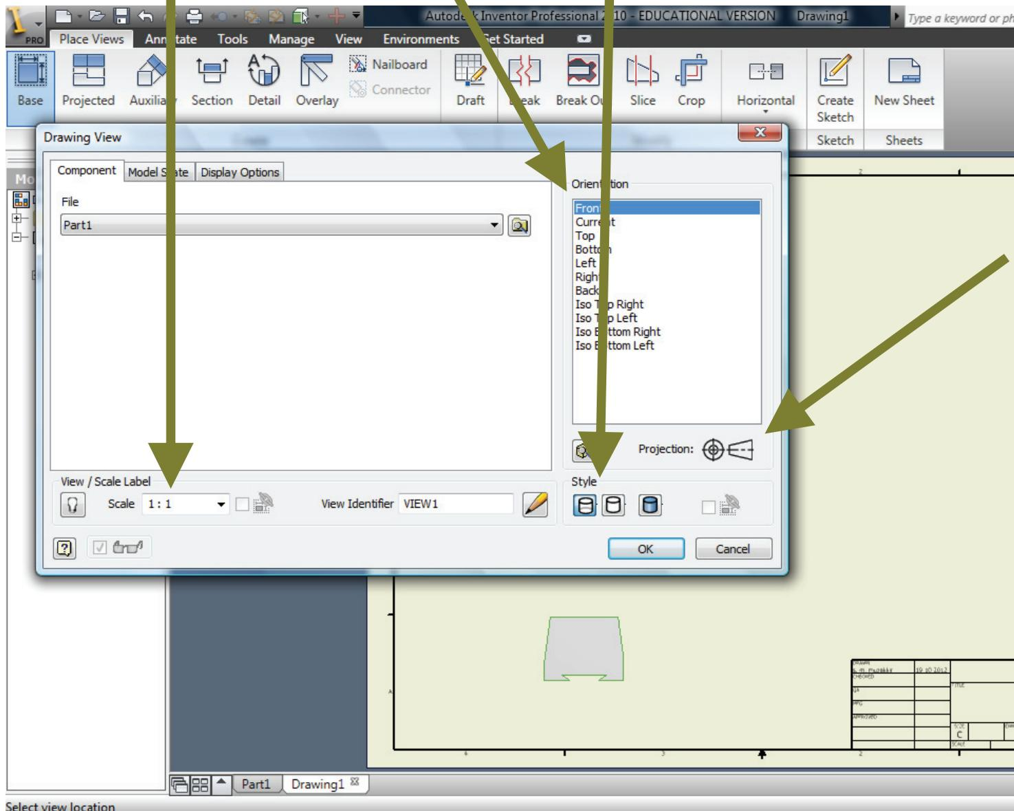
Note the III angle projection method, default for ANSI drawing
