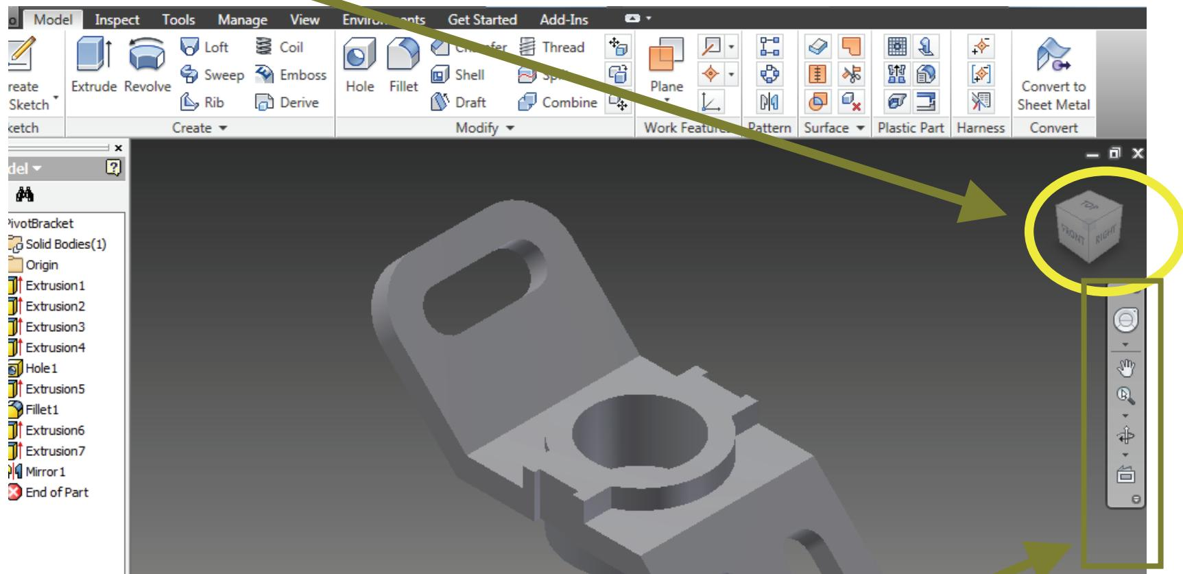
The tools on the **Navigation Bar** helps to control the view and orientation of components in the drawing window
