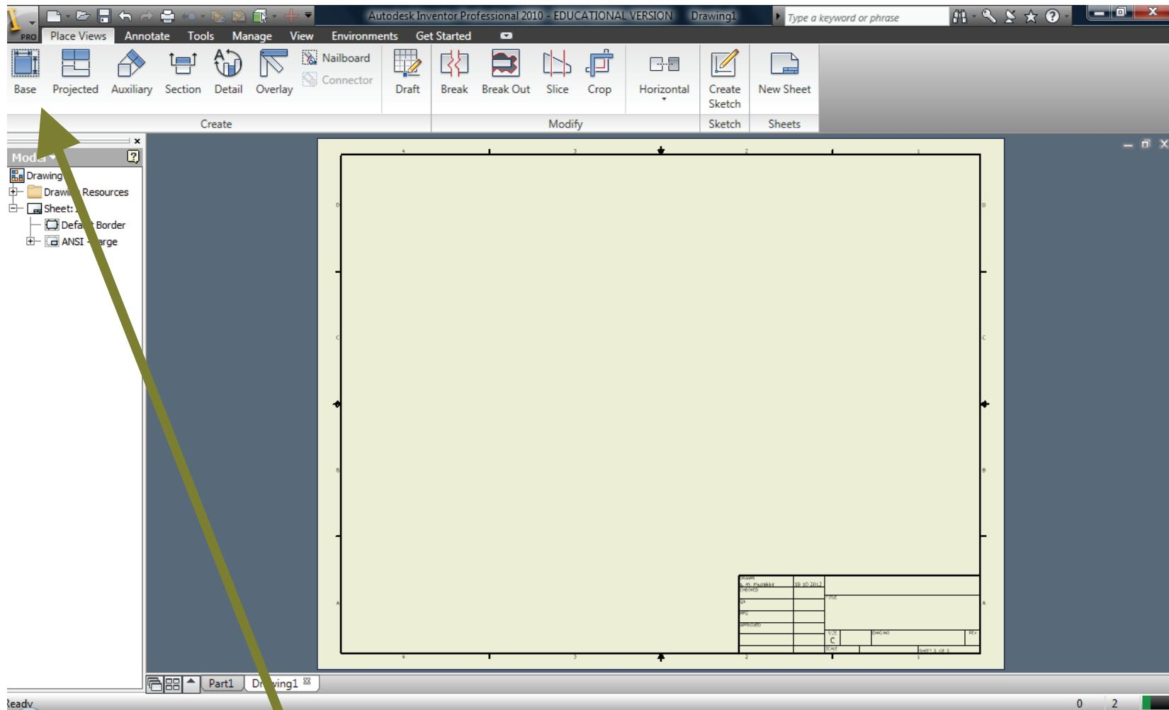
Now activate the **Base** command to insert the solid model whose orthographic projections is required.
